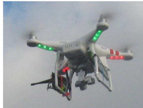
Fig. 7. Quadcopter with the radio payload
