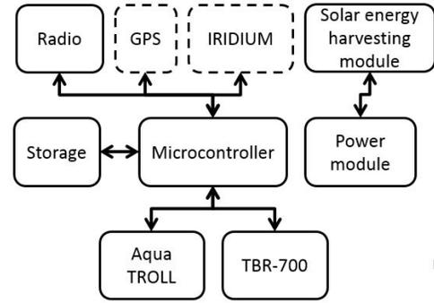
Fig. 2. The floating node hardware architecture
