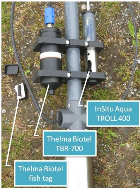
Fig. 4. TBR-700 (left) and Aqua TROLL (right) sensors integrated with buoy
