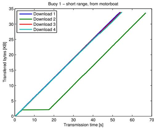
Fig. 8. Buoy 1 - short range communication, motorboat relay
