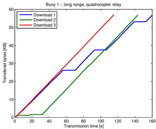
Fig. 12. Buoy 1 - long range communication, quadcopter relay
