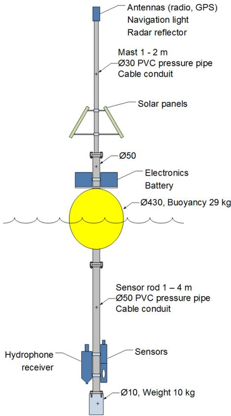
Fig. 1. Overall buoy design
