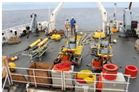
Fig 3. CMRE equipment on the NRP Gago Coutinho. eFolaga vehicles are shown on the left, the two Wave Gliders on the right. The Wave Rider buoy is shown behind the rightmost Wave Glider.
