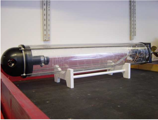
Fig. 2. The Skarv AUV. Here one can clearly see the bow thruster and rear propeller and control planes. The AUV is here shown without control hardware and batteries.
