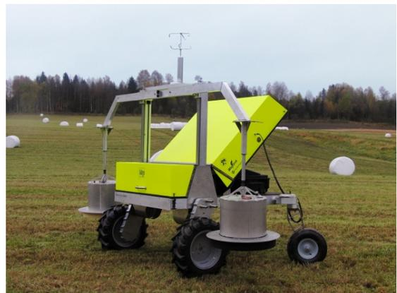
Fig. 1. A robot developed for autonomous N<sub>2</sub>O measurements on cereal fields. The robots autonomy is currently under development where efficient attitude estimation is a focus.
