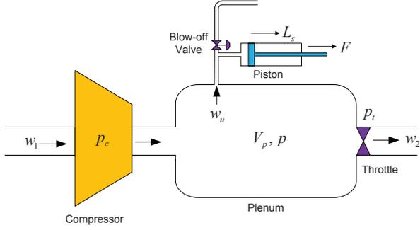
Fig. 1. Compression system equipped with a piston.
