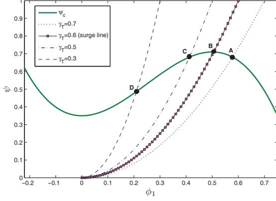
Fig. 2. Compressor and throttle characteristics.
