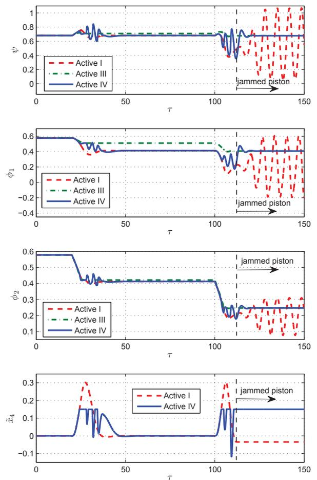
Fig. 7. Compressor states and piston stroke in a condition where the pistons of Active I and Active IV are jammed at  $\tau = 112$ .
