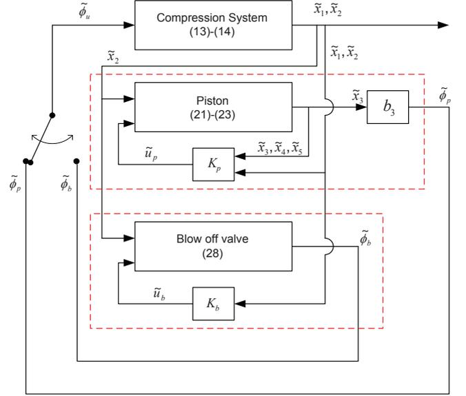
Fig. 3. Control diagram with switching operation of active surge control with piston actuation and blow off valve.
