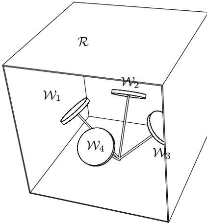
Fig. 1. Illustration of a gyrostat with four reaction wheels in a tetrahedron configuration.
