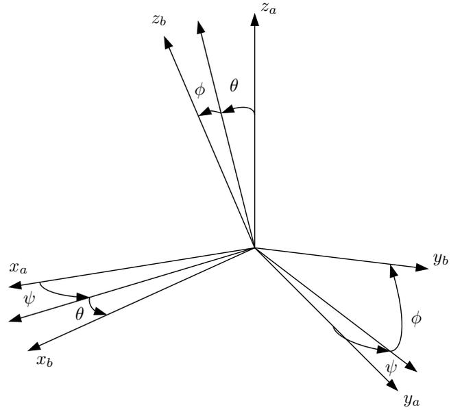
Fig. 2. The figure illustrates how rotation between two frames can be interpreted in form of Euler angles.
