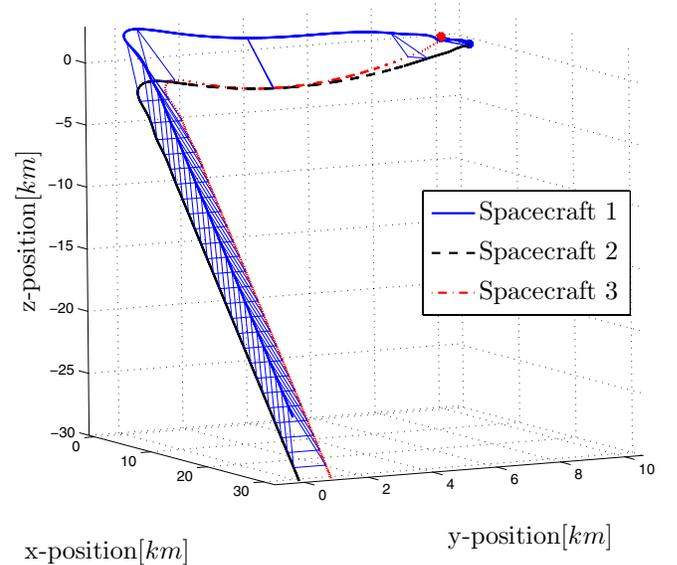
Fig. 4. Tracking and synchronization behaviour in position. All units are in km. The triangles indicate the relative position at different time-instants. The initial position is indicated by a \*.
