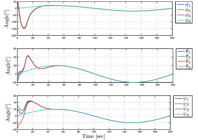
Fig. 3. The figure illustrates how the attitudes of the three spacecraft are first mutually synchronized, and then track a desired orientation.
