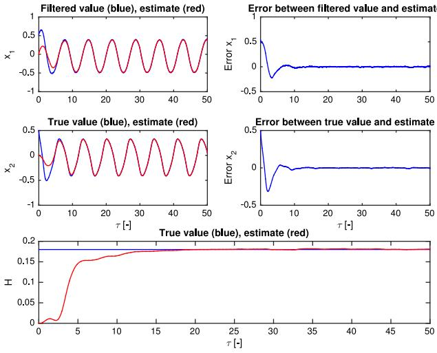
**Fig. 4.** Real (blue) and estimated (red) states  $x_1$ ,  $x_2$  and  $H$  for the best obtained minima (closest to real values) of  $W$  and  $B$  for the filtered measurement signal.
