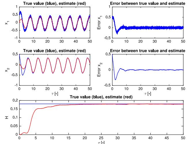
**Fig. 2.** Real (blue) and estimated (red) states  $x_1$ ,  $x_2$  and  $H$  for the obtained minima (closest to real values) of  $W$  and  $B$  for added measurement noise.
