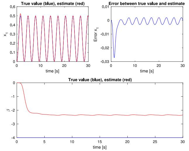
**Fig. 6.** True value and estimate of state  $x_1$  together with their error as well as true value and estimate of parameter  $\beta$ .
