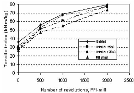
Figure 7 - Tensile index as a function of revolutions in a PFI mill. The heat pump dried pulps are compared to mill dried
