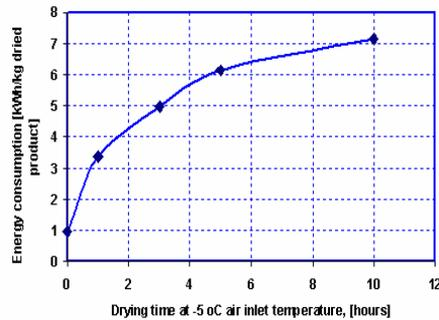
Figure 8: *Dryer energy consumption per kg dried cod pieces with increasing time at  $-5^{\circ}\text{C}$*
