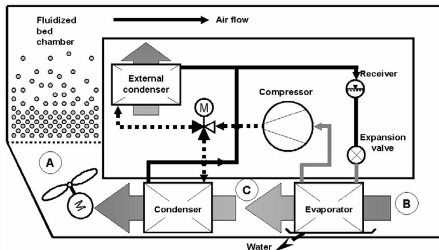
Figure 1 Schematic layout of a fluid bed dryer with heat pump
