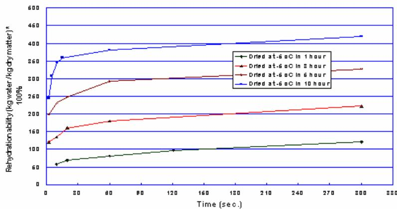
Figure 4. Rehydration ability of cod pieces dried with different time periods at freeze drying conditions
