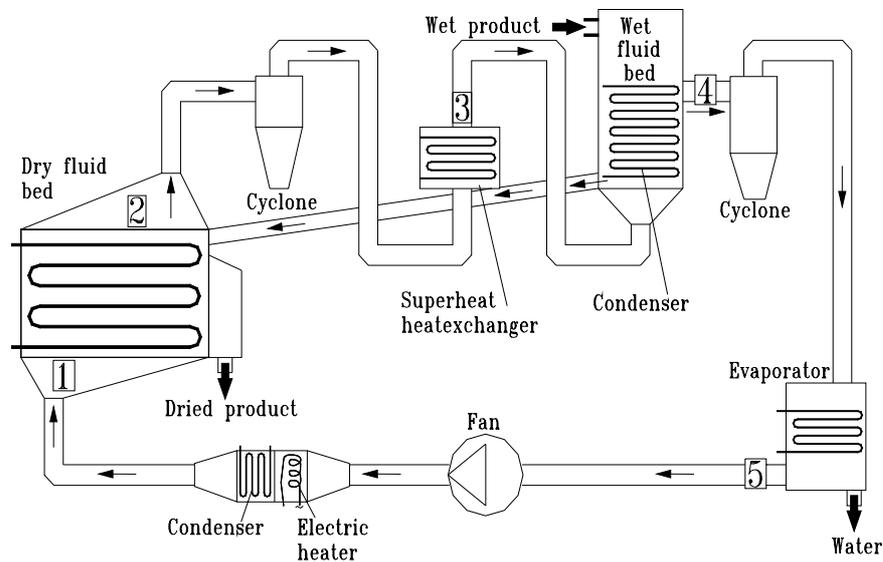
Figure 2. Nonadiabatic, two-stage, plug-flow  $\text{NH}_3$  heat pump fluid bed dryer
