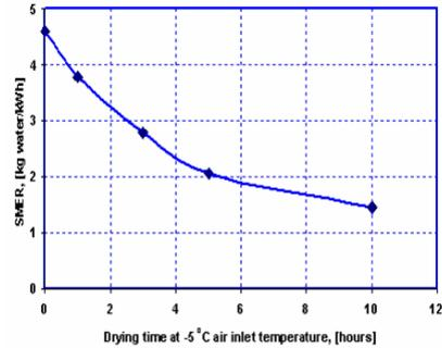
Figure 9: *SMER for dried pieces of cod with increasing drying time at  $-5^{\circ}\text{C}$*
