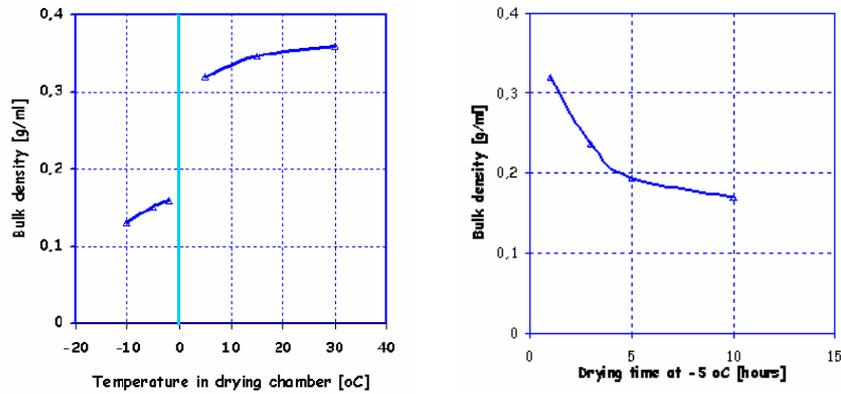
Figure 3. Bulk density of cod pieces dried at temperatures from  $-10^{\circ}\text{C}$  to  $30^{\circ}\text{C}$
