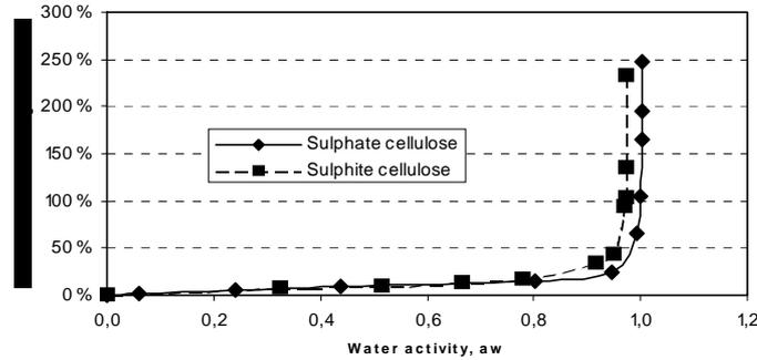
Figure 4 - Sorption isotherms for sulphate and sulphite cellulose
