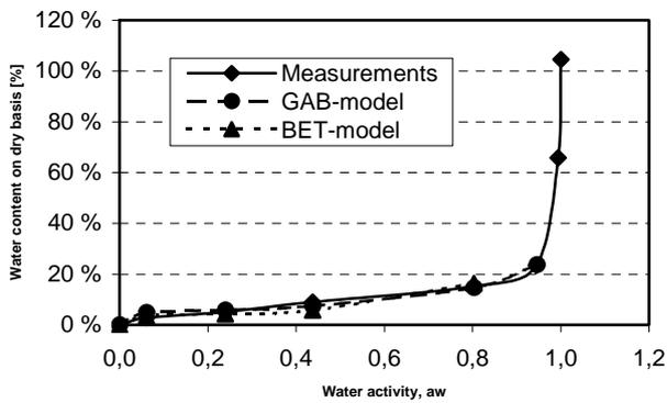
Figure 7 - Experimental and GAB/BET model sorption isotherm for sulphate
