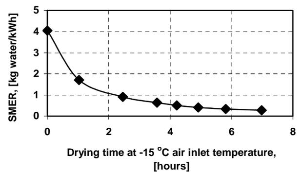
Figure 10 – SMER for dried sulphate cellulose with increasing drying time at low temperature
