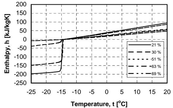
Figure 6 - Specific enthalpy of sulphite cellulose at different water content on wet basis
