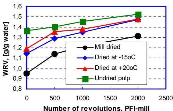
Figure 2 - Water retention value as a function of revolutions in a PFI mill. The heat pump dried pulps are compared to mill dried and never dried pulps.
