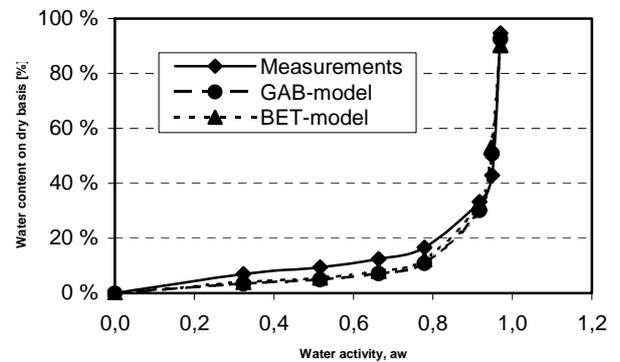
Figure 8 - Experimental and GAB/BET model sorption isotherm for sulphite
