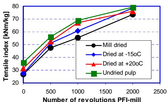
Figure 3 - Tensile index as a function of revolutions in a PFI mill. The heat pump dried pulps are compared to mill dried and never dried pulps.
