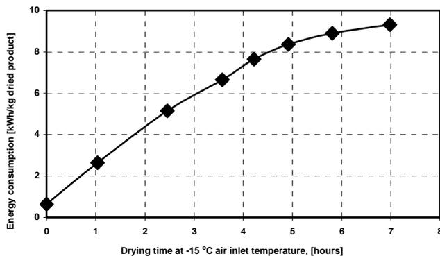
Figure 9 – Dryer energy consumption per kg dried sulphate cellulose with increasing drying time at low temperature
