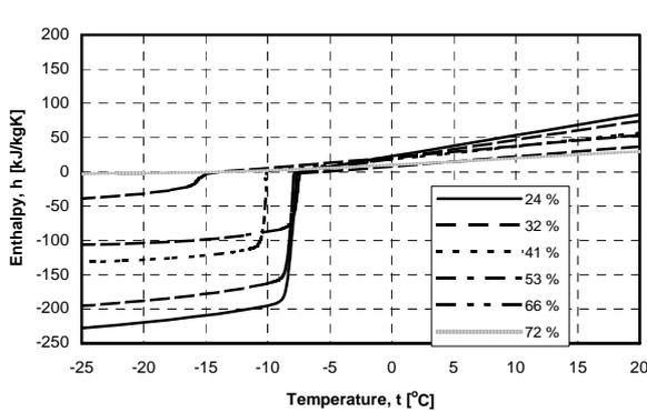
Figure 5 - Specific enthalpy of sulphate cellulose at different water content on wet basis
