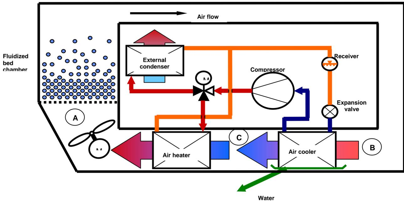
Figure 1 – Schematic layout of a heat pump fluidized bed dryer
