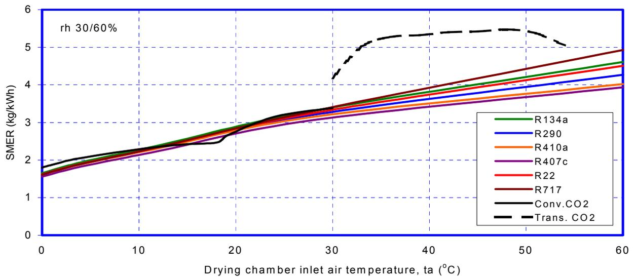
Figure 4. SMER as function of air temperature for different working fluids and CO<sub>2</sub> at conventional and transcritical cycles
