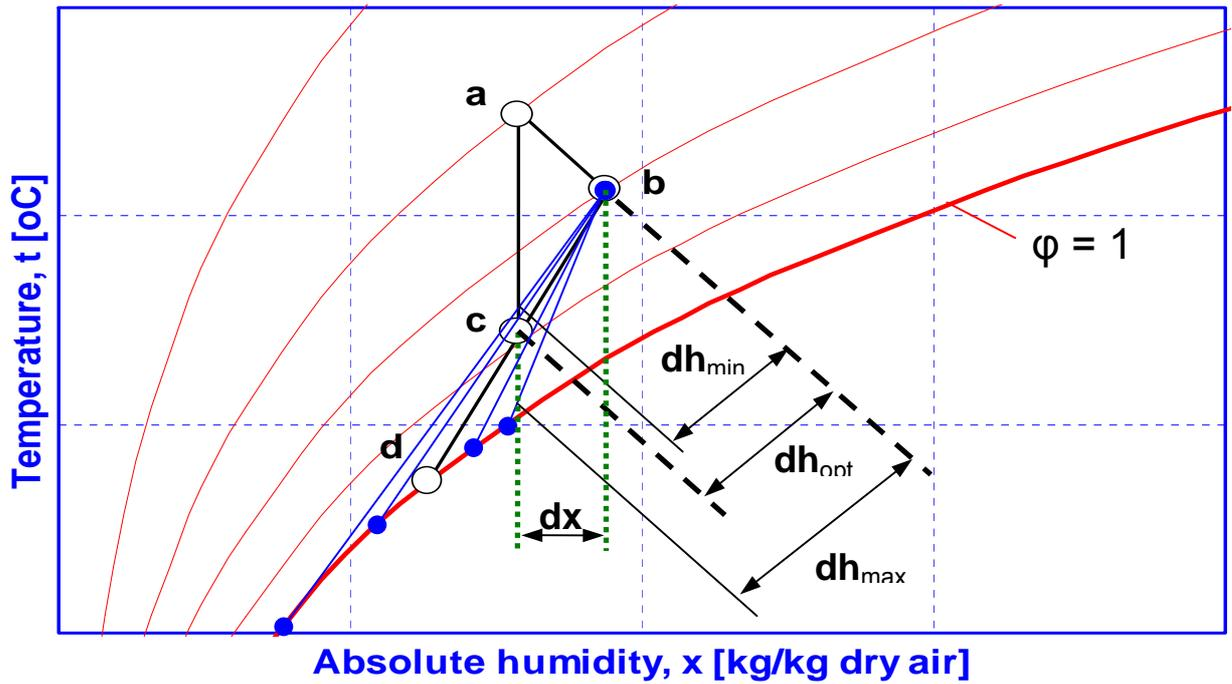
Figure 2. Mollier chart for humid air with heat pump drying process state points
