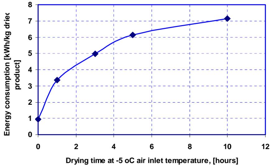
Figure 8: Dryer energy consumption per kg dried cod pieces with increasing time at  $-5^{\circ}\text{C}$
