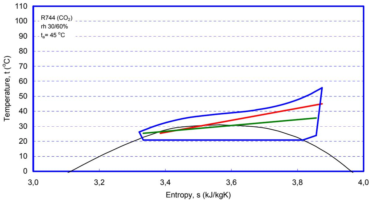
Figure 3. Temperature-entropy diagram for the heat pump dryer with carbon dioxide in transcritical cycle
