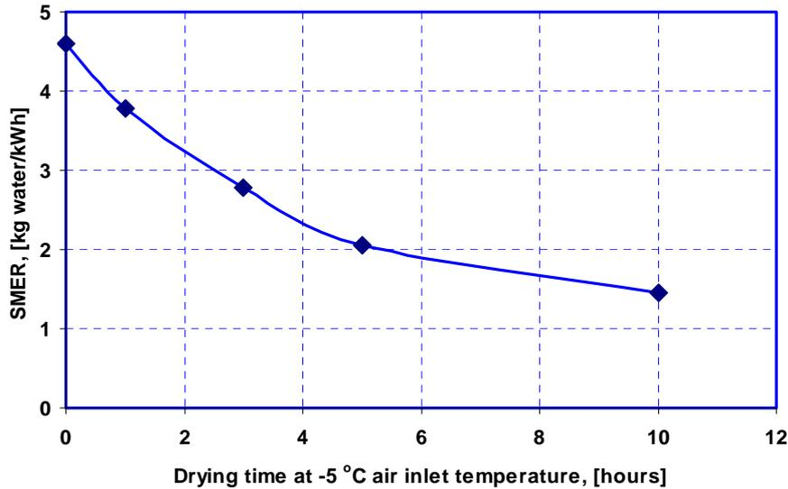
Figure 9: SMER for dried pieces of cod with increasing drying time at –5°C
