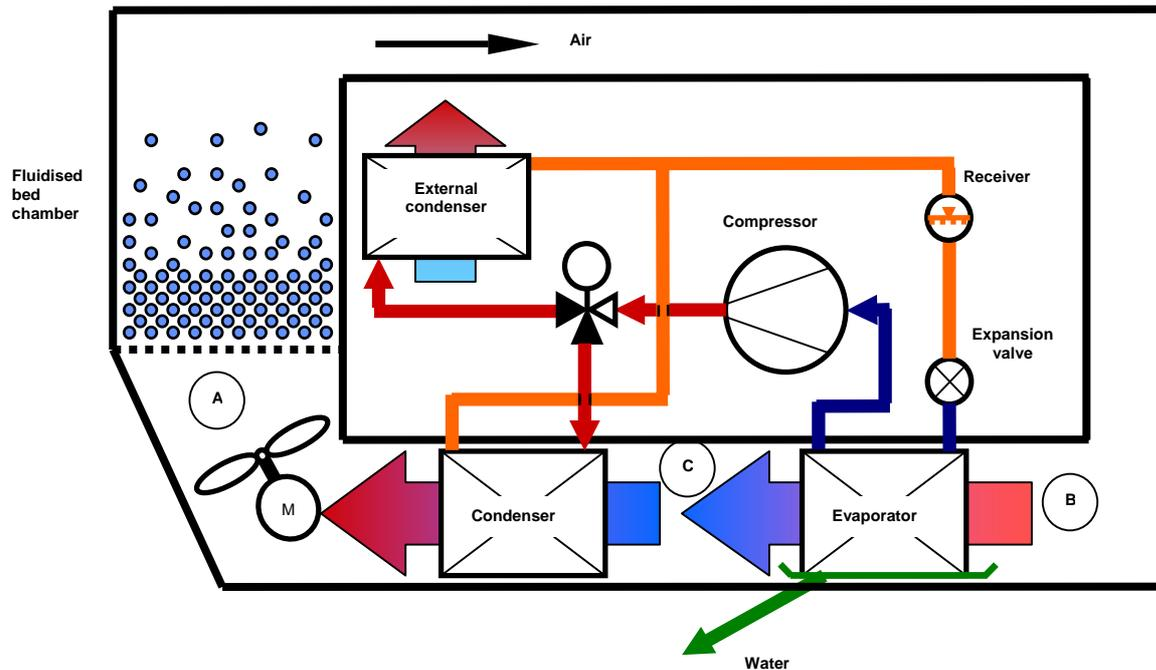
Figure 1. Schematic layout of a heat pump fluidized bed dryer
