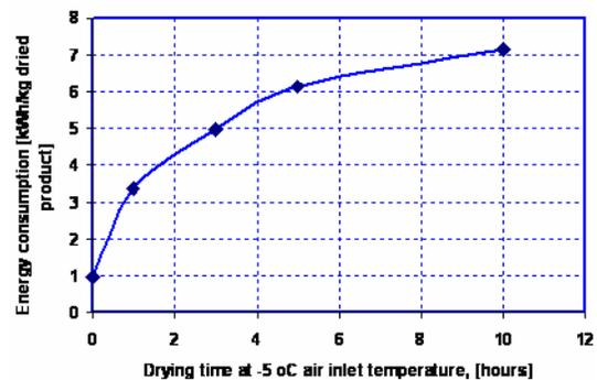
**Figure 11:** Dryer energy consumption per kg dried cod pieces with increasing time at low temperature
