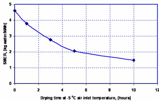
**Figure 10:** SMER for dried pieces of cod with increasing drying time at low temperature
