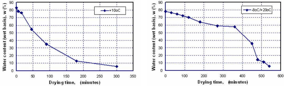
**Figure 3** Drying curves for the cod pieces with drying temperature at +10°C and with start temperature program at -8°C and final drying at +20°C
