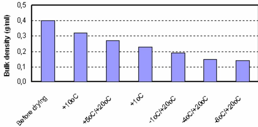
**Figure 5:** Bulk density of cod pieces dried at different temperature programs
