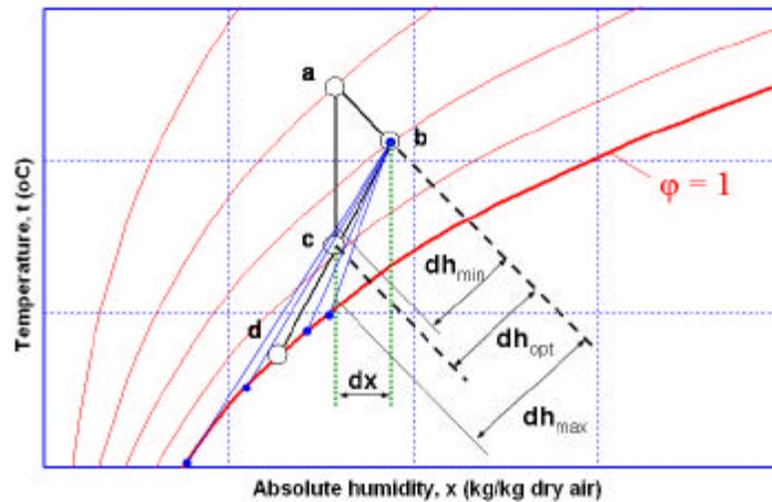
**Figure 2** Mollier diagram for the drying process
