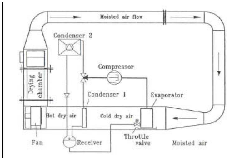
**Figure 1** Layout of the fluid bed heat pump dryer
