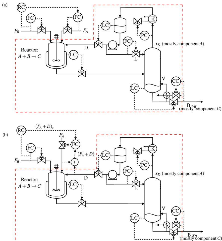
**Figure 11.** Reactor–recycle system with two reactants (A + B). (a) Inconsistent structure with both reactant flows given. (b) Local-consistent structure where feed of reactant A depends on inventory of A (as reflected by the recycle D).
