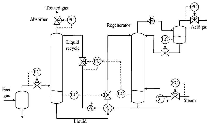
**Figure 8.** Absorber and regenerator example: not consistent liquid inventory control.
