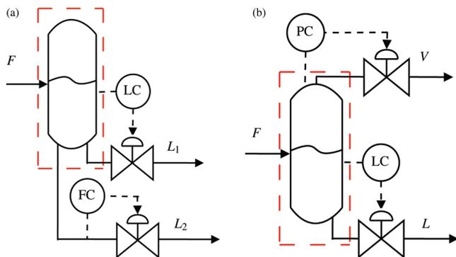
**Figure 4.** Local-consistent inventory control of split with one and two phases. (a) Single-phase tank: adjustable split. (b) Two-phase tank: inventory control determines split.
