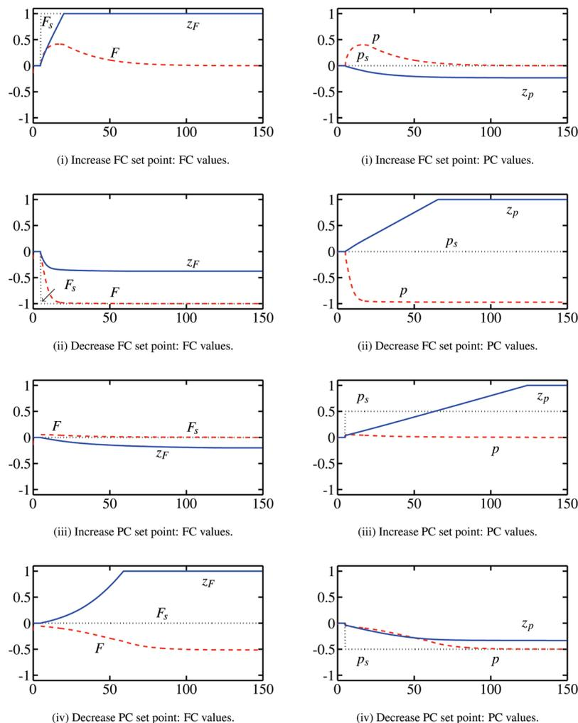
**Figure 2.** Dynamic simulations of inconsistent configuration in Figure 1d. Left column: flow controller (FC). Right column: pressure controller (PC). In all cases, one of the two valves moves to fully open.  $z_F$ , inlet valve opening (from  $-1$  to  $1$ );  $z_p$ , outlet valve opening.
