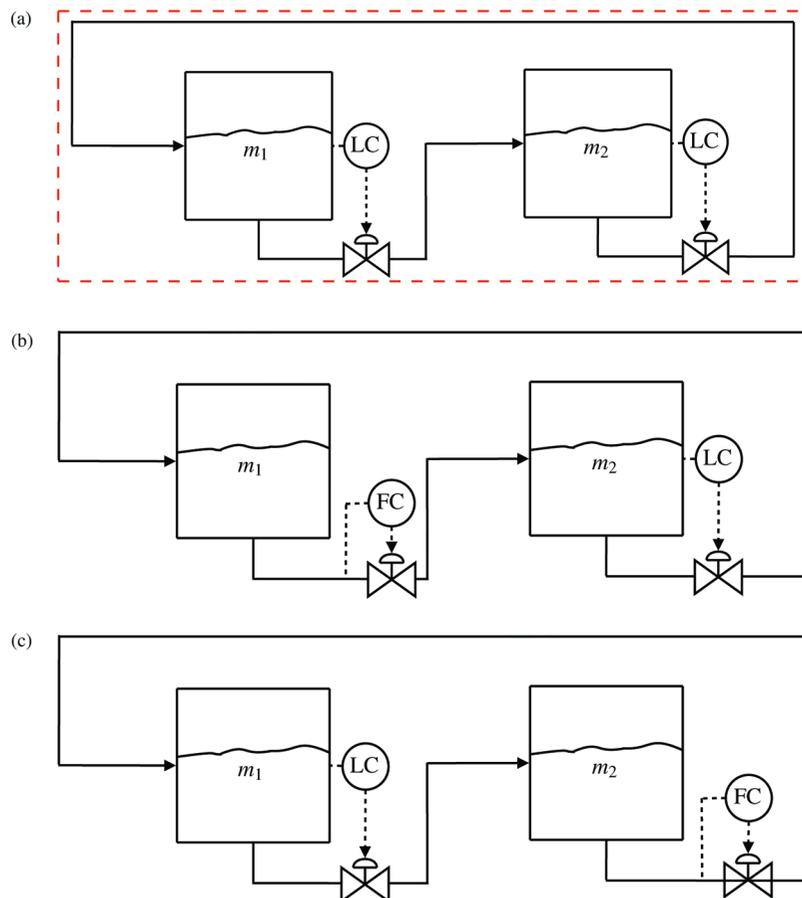
**Figure 7.** Inventory control for closed system. (a) Not consistent (because there is no uncontrolled inventory). (b) Local consistent (inventory  $m_1$  is uncontrolled). (c) Local consistent (inventory  $m_2$  is uncontrolled).
