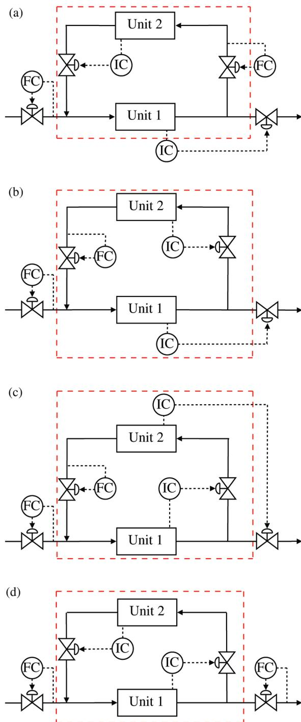
**Figure 6.** Inventory control of simple recycle process with given feed. (a) Local-consistent inventory control. (b) Local-consistent inventory control. (c) Consistent, but not local-consistent inventory control. (d) Not consistent inventory control.
