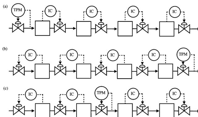
**Figure 5.** Local consistency requires a radiating inventory control around a given flow (TPM). (a) TPM at inlet (feed): inventory control in direction of flow. (b) TPM at outlet (on demand): inventory control in direction opposite to flow. (c) General case with TPM inside the plant: radiating inventory control.
