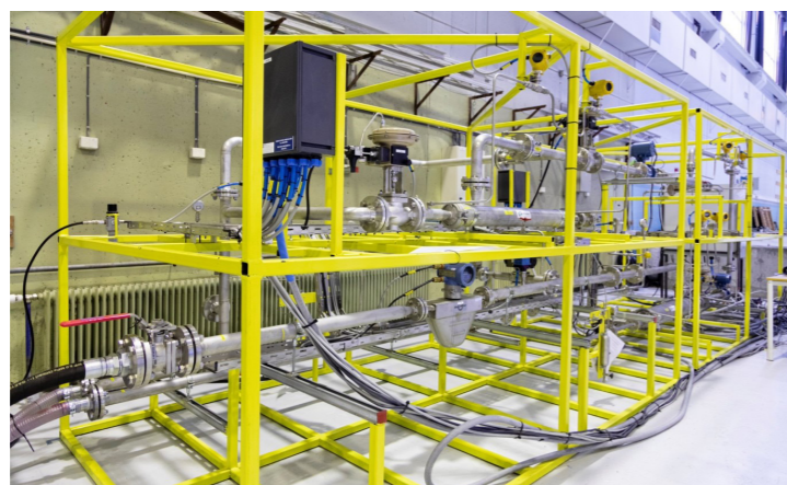
Figure 5: SUBPRO Compact separation lab for testing control algorithms
