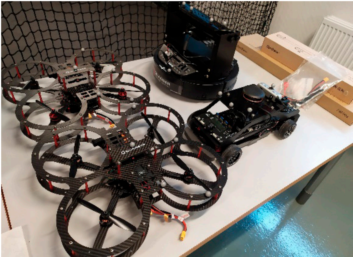
Figure 1: drones, vehicles, and robots in the autonomous vehicle research studio. They are equipped with embedded computers, cameras and sensors that enable the sensing of operation environment and network communication.
