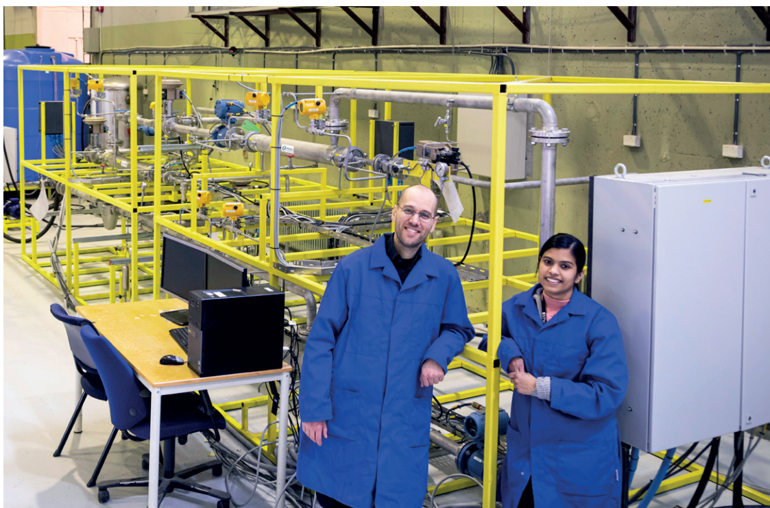
Figure 3: Hydrocyclone test rig with pump and tank system. PhD student Mishiga Vallabhan and her project manager and main supervisor Associate Professor Christian Holden.
