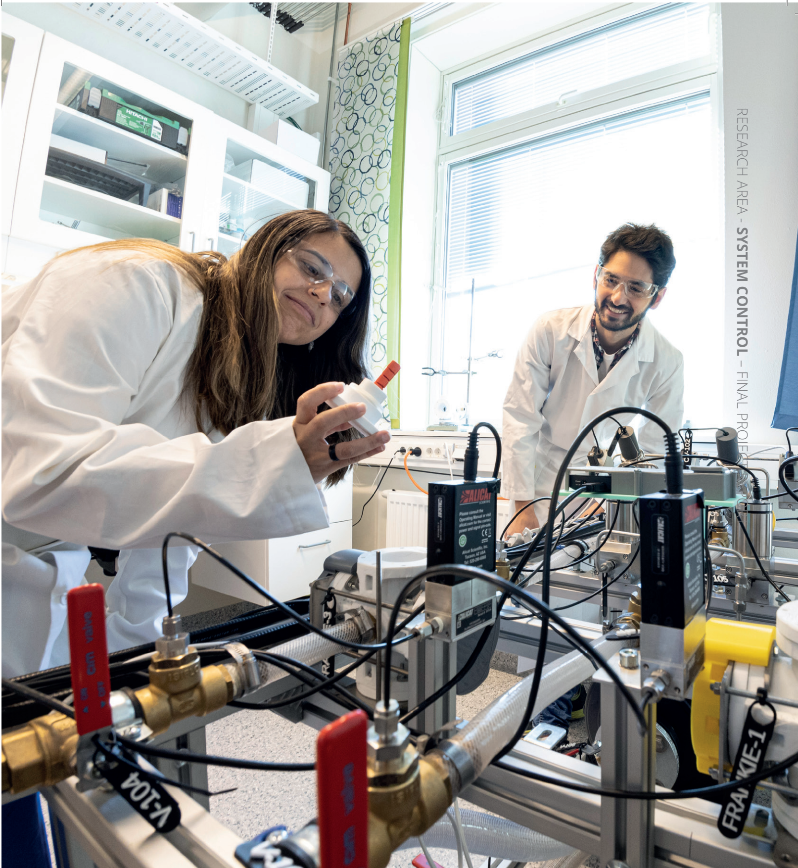
Figure 5: From left to right: associate PhD student Allyne dos Santos (Faculty of Natural Sciences NTNU) and Postdoctoral fellow Jose Otavio Assumpcao Matias working on the lab rig developed in this project for testing the health-aware controller and control approaches for gas-lift optimization.
