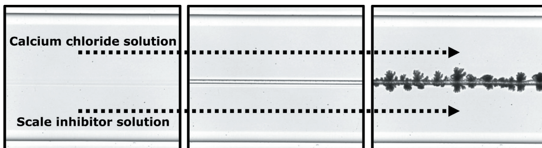
Timelapse of a microfluidic precipitation of calcium – scale inhibitor complex. Laminar flow in the channels allows for a stable water-water interface and diffusion across it, favouring controlled crystallization process.
