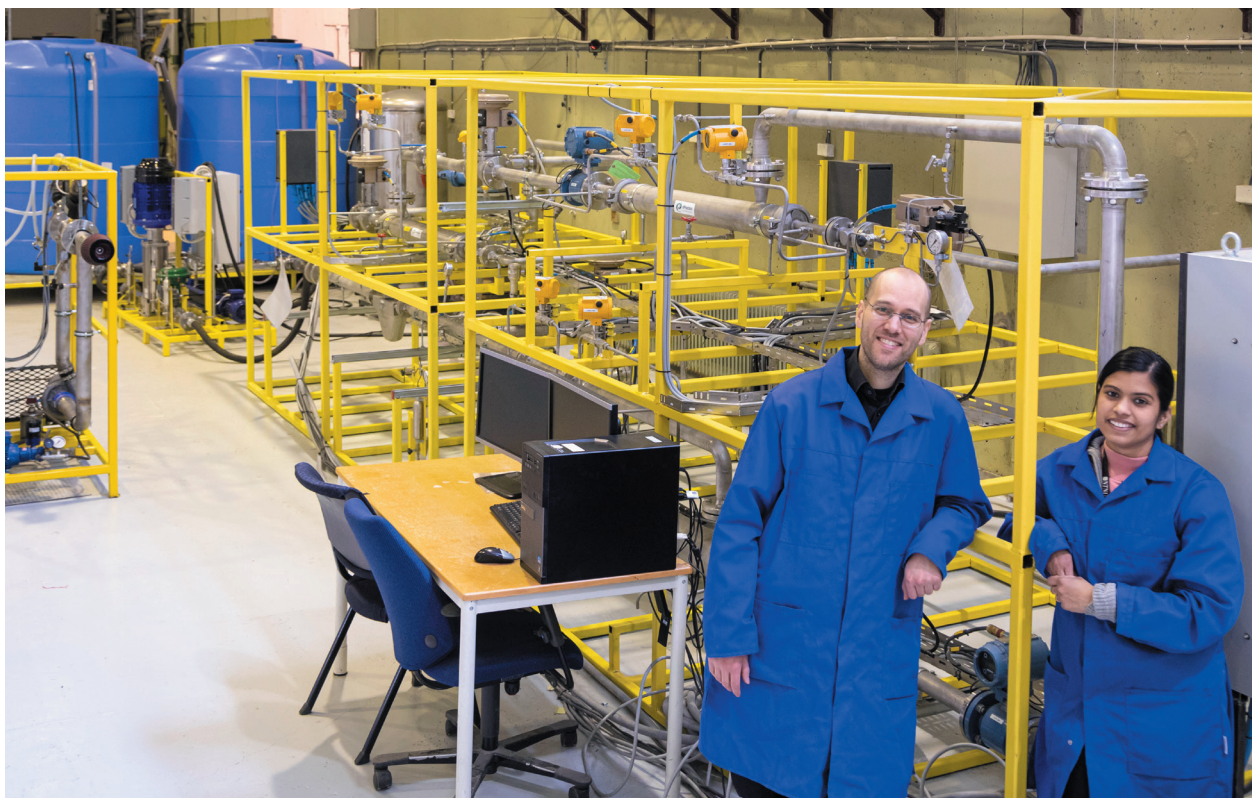
Hydrocyclone test rig with pump and tank system. PhD student Mishiga Vallabhan and her project manager and main supervisor Associate Professor Christian Holden
