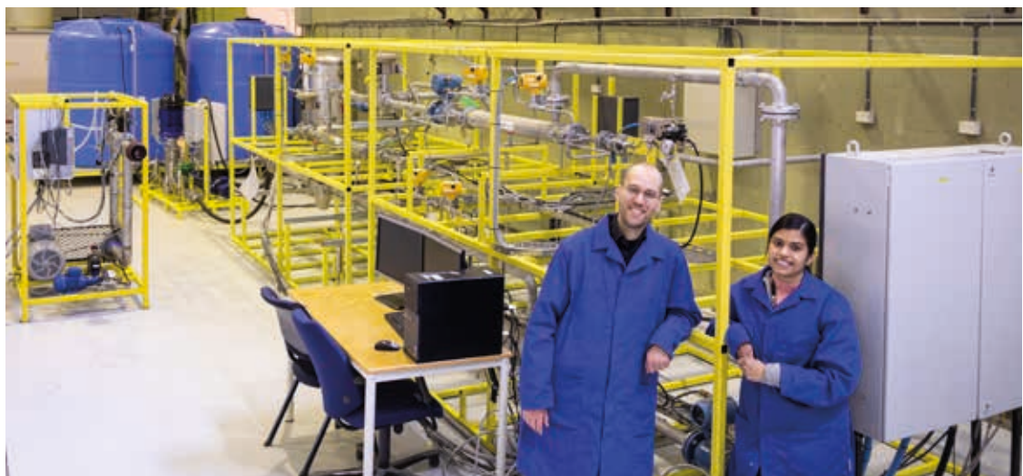
Hydrocyclone test rig with pump and tank system.
