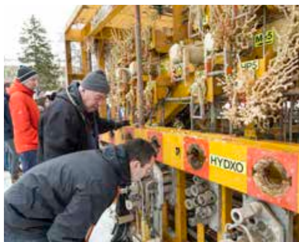
This is from an excursion to Statoil at Rotvoll, to take a closer look at two Subsea Distribution Units from the Njord-field. The SDU's subsea units have been in uninterrupted operation subsea since 1997, in symbiosis with the deep sea corals!
