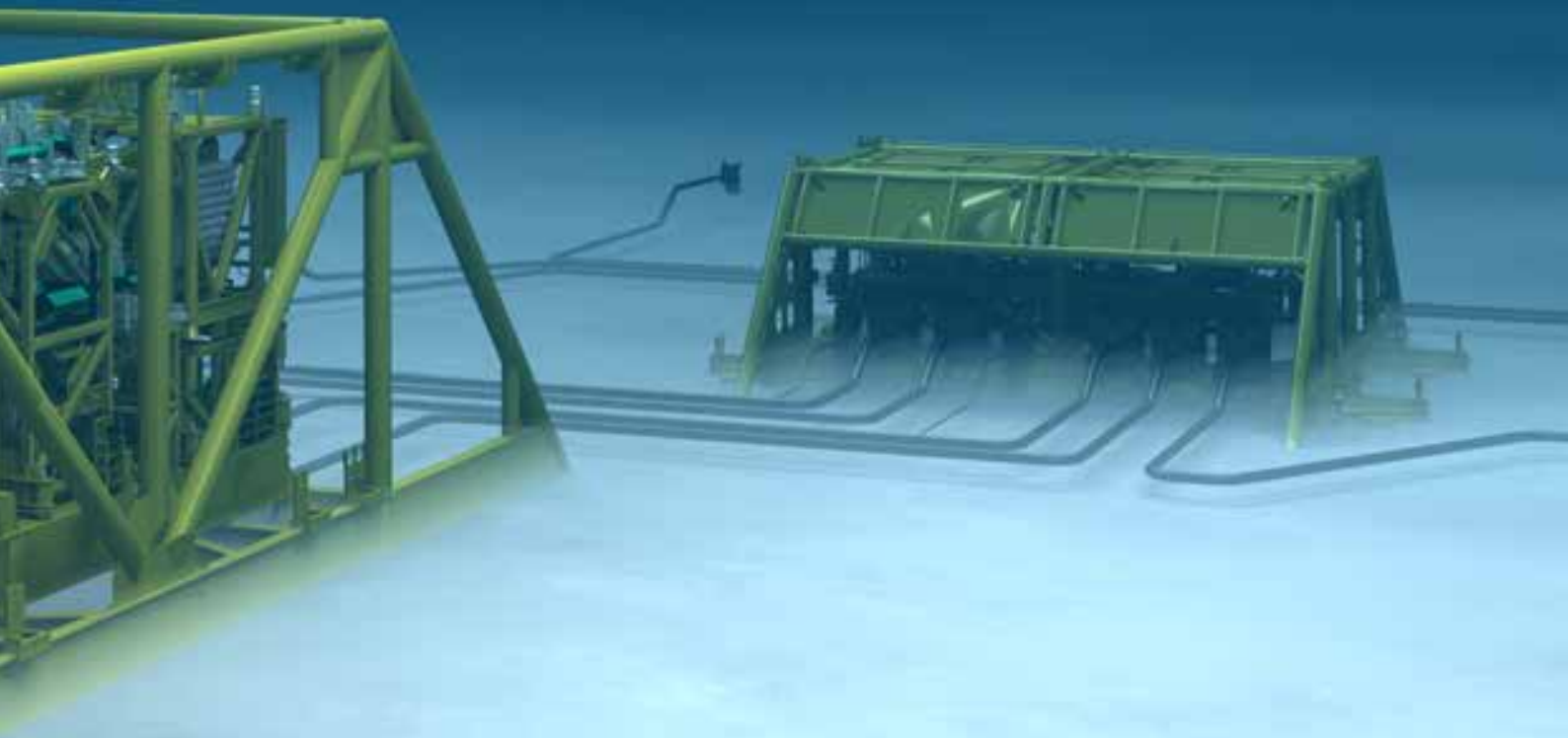
Åsgard subsea compression system, courtesy of Statoil.
