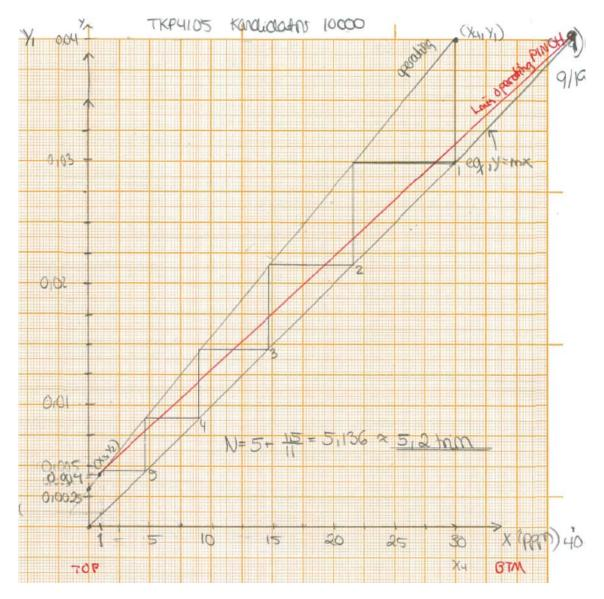
Comment 1: As mentioned, the "exact" McCabe-Thiele diagram should start from (x3,y2)=(1.e-6,0.00417) instead of (1.e-6,0.004). In addition, the operating line will curve a little upwards. Both these effects give a slight reduction in the "exact" number of stages; see also Example 10.6-2 in the book for how to make curved operating lines.
