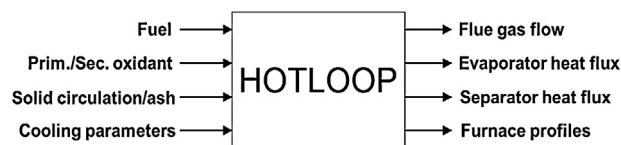
Fig. 3. Simplified input–output structure of the hotloop model.
