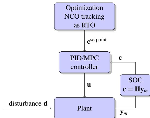
Figure 5.5: Relation between NCO tracking and self-optimizing control
