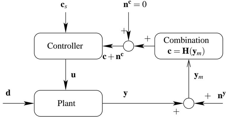
Figure 3.3: Control structure (with integral action,  $\mathbf{c}_s = \mathbf{c}$  at steady state,  $\mathbf{n}^c = 0$ ), (Adapted from [Alstad et al., 2009])
