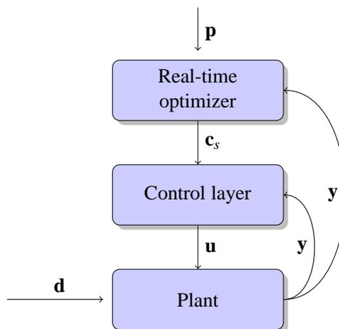
Figure 2.3: Conventional RTO scheme.  $\mathbf{d}$ : external disturbance,  $\mathbf{p}$ : prices,  $\mathbf{u}$ : input,  $\mathbf{y}$ : measurements.
