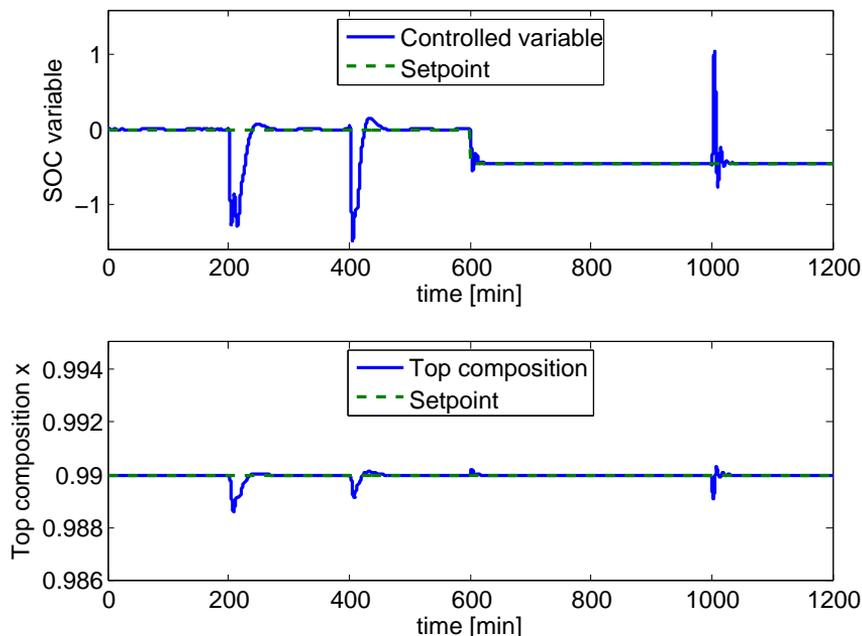
Figure 3.9: Controlled variables: Self-optimizing controlled variable and top composition
