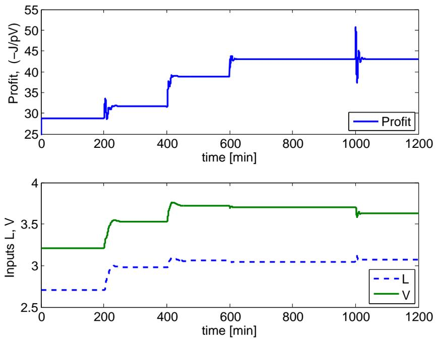
Figure 3.8: Profit and inputs for the distillation column
