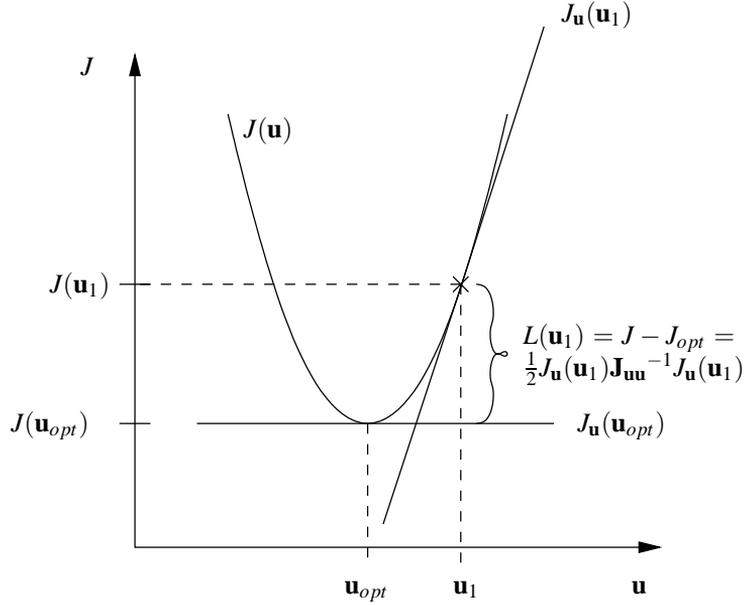
Figure 3.4: Loss  $L$  imposed by non-optimal operation
