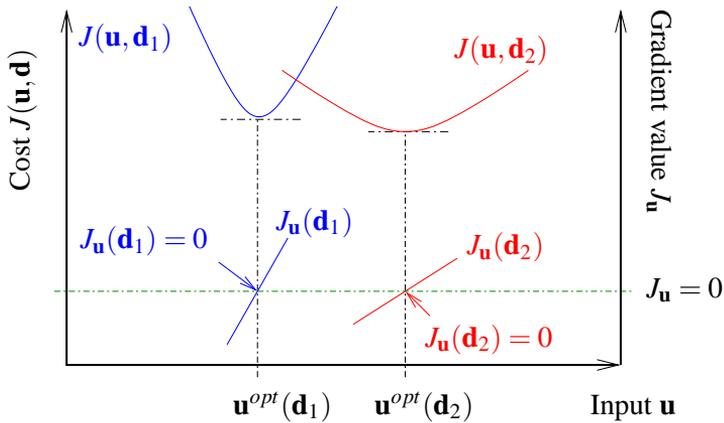
Figure 3.1: Cost and gradients for different disturbances  $\mathbf{d}$
