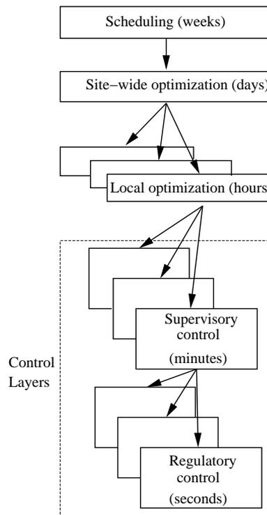
Figure 2.1: Hierarchical control structure [Skogestad, 2000a]
