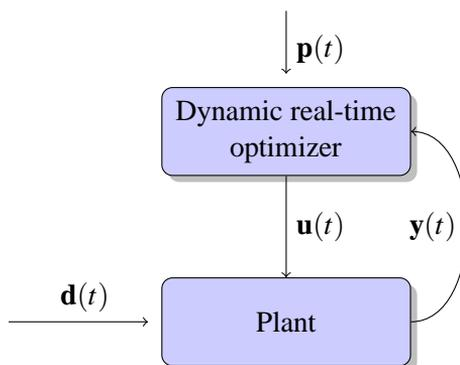
Figure 2.2: Dynamic RTO scheme.  $\mathbf{d}(t)$ : external disturbance,  $\mathbf{p}(t)$ : prices,  $\mathbf{u}(t)$ : input,  $\mathbf{y}(t)$ : measurements.
