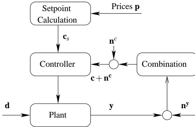
Figure 3.5: Feedback control structure with setpoint calculation (with integral action,  $\mathbf{n}^c = 0$ )
