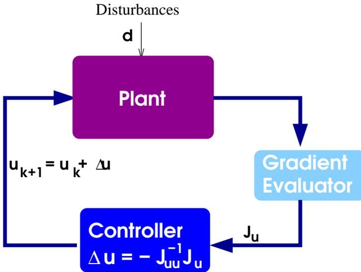
Figure 5.2: Block diagram NCO tracking
