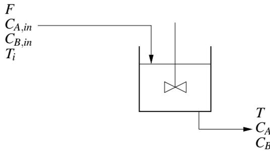
Figure 5.6: Schematic diagram of a CSTR
