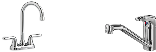
(a) Traditional design with two separate handles ( u_1 = F_1, u_2 = F_2 ) (b) Modern one-handle design where decoupling is achieved by the physical design ( v_1 = F_1 + F_2 and v_r = \frac{F_1}{F_2} ).
