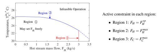
Figure 2: Active constraint regions for the cooler
