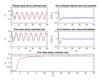
Fig. 6. Real (blue) and estimated (red) states  $x_1$ ,  $x_2$  and H for the best obtained minima of W and B for the filtered measurement signal.
