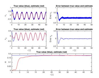
Fig. 4. Real (blue) and estimated (red) states  $x_1$ ,  $x_2$  and H for the best obtained minima of W and B for added measurement noise.
