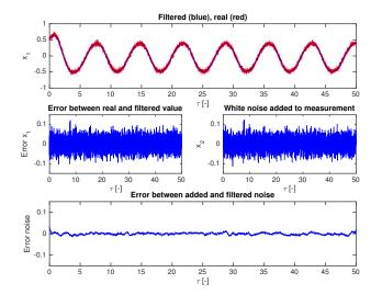
Fig. 7. Real and filtered state  $x_1$  and residual noise
