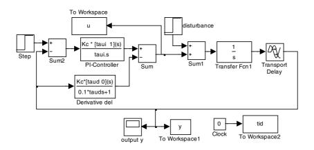
Figure 3-2 Block diagram for parallel control system in Simulink®..
