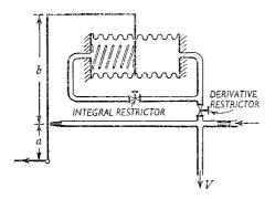
Figure 2-4 Series/Cascade -coupled PID-controller
