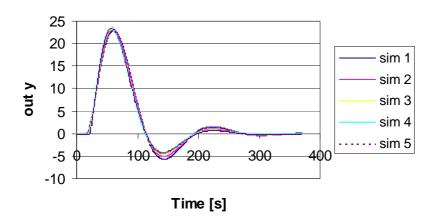
Figure 3-5 Process simulation results for PI-Controller
