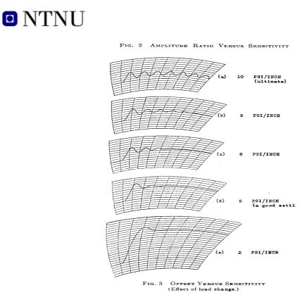
Figure 2-1 Offset versus sensitivity. Effect of load change.
