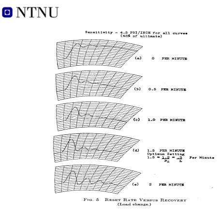
Figure 2-2 Reset-rate versus recovery. Load change.
