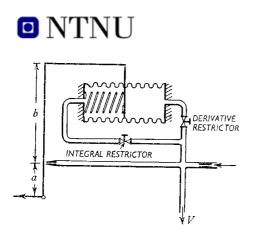
Figure 2-5 Parallel-coupled pneumatic PID-controller
