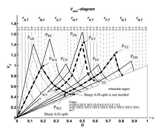
Figure 6: Assessment of minimum vapour flow for separation of a 8-component feed (ABCDEFGH) into 4 products (WXYZ). The plot shows the  $V_{min}$ -diagram for the feed components (solid) and the equivalent diagram for the products (bold dashed) is easily obtained from the product split specifications given in Tables 2 or 3.
