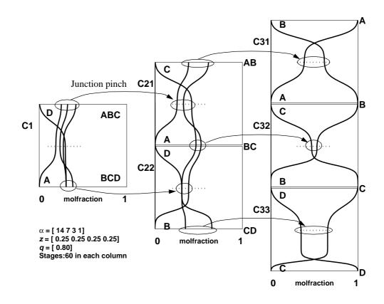
Figure 5: Composition profiles for the Petlyuk arrangement in Figure 1. Each column is operated at its preferred split with vapour flows and product splits taken from Table 1 data as shown in the  $V_{min}$ -diagram in Figure 4. Observe the pinch zones in all junctions and how one component is removed in each column end.
