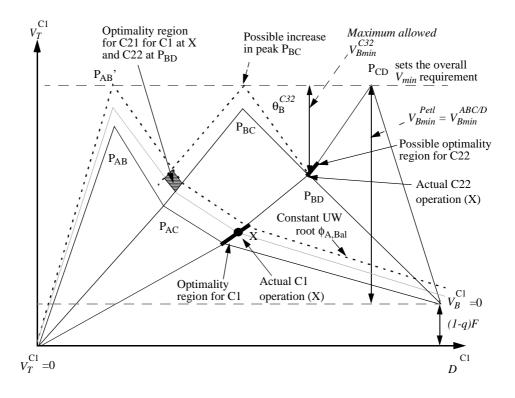
Figure 7:  $V_{min}$ -diagram for 4-component feed ABCD with optimality regions for operation of columns C1, C21 and C22. The contour lines for constant  $\phi_A$  and a given constant  $\theta_B^{C2I}$  which makes  $V^{A/BCD} = V^{AB/CD} = V^{ABC/D}$  are shown (dashed). These boundaries are the upper bounds for the optimality regions.
