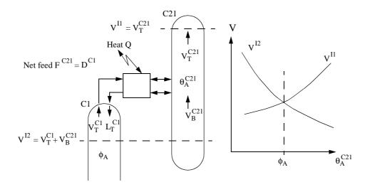
Figure 8: General column interconnection junction. The direct (full thermal) coupling gives  $\theta_A^{C2I} = \phi_A$  which implies  $min(max(V^{II}, V^{I2}))$  and a zero external heat exchange at the interconnection (Q=0).
