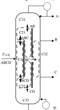
Figure 9: Practical 4-product Petlyuk arrangements with some flow restrictions: We allow only liquid feed to C32 and liquid intermediate side products B and C.
