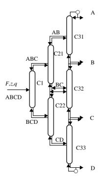
Figure 1: The Petlyuk arrangement extended to four products. Vapour and liquid flow rates can be set individually in each internal 2-product column.
