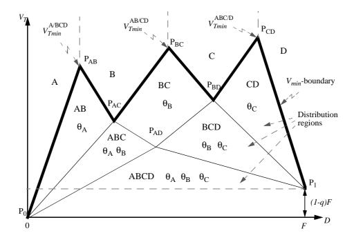
Figure 2:  $V_{min}$ -diagram for a given 4-component feed (ABCD) to the prefractionator. The set of distributed components and corresponding active Underwood roots are indicated in each distribution region. The preferred split is at  $P_{\rm AD}$ .
