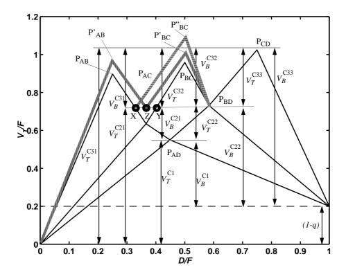
Figure 10:  $V_{min}$ -diagram for 4-component feed ABCD with the less flexible Petlyuk arrangement in Figure 9. Vertical arrows are vapour flow requirements in each column section. Feed data:  $z=[0.25\ 0.25\ 0.25\ 0.25\ 0.25],\ \alpha=[14,7\ ,3,1],q=0.8$
