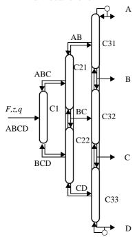
b) Implemented in a single shell as a dividing wall column (DWC)
