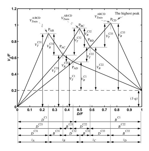
Figure 4:  $V_{min}$ -diagram showing the minimum vapour flows and product splits for every section in the Petlyuk arrangement in Figure 1 when each column C1, C21 and C22 operates at its preferred split (note that the subscript min should be on every vapour flow).
