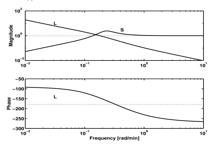
Bandwidth  $\omega_B$ : Frequency up to which control is effective Closed loop response time  $\tau_c \approx 1/w_B$
