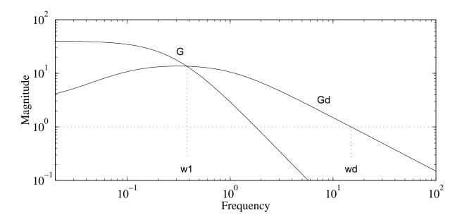
Input saturation is expected for disturbances at intermediate frequencies from  $\omega_1$  to  $\omega_d$  A buffer tank may be added to reduce the effect of a disturbance. It reduces the distrurbance effect at frequencies above  $1/t_{buffer}$ .
