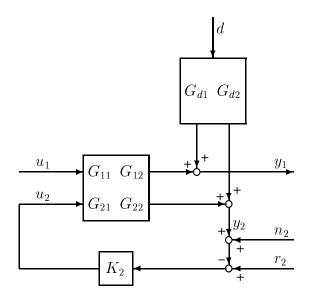
Figure 7: Block diagram of a partial control system
