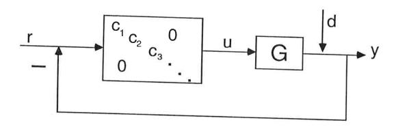
Fig. 1 Decentralized control structure.
