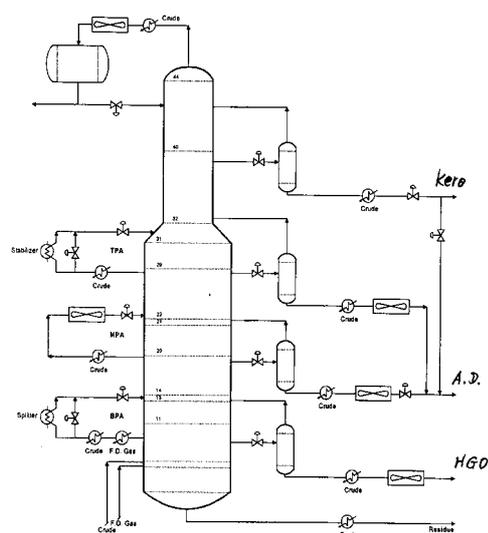
Figure 4.1 Simplified flow diagram of crude unit atmospheric distillation column
