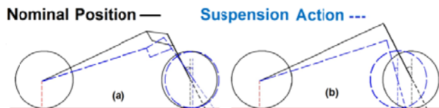
Figure 3. a) Duolever suspension system, head angle trail and wheelbase increase with the travel of the suspension. b) Telescopic fork suspension. Head angle, trail and wheelbase decrease with the travel of the suspension.
