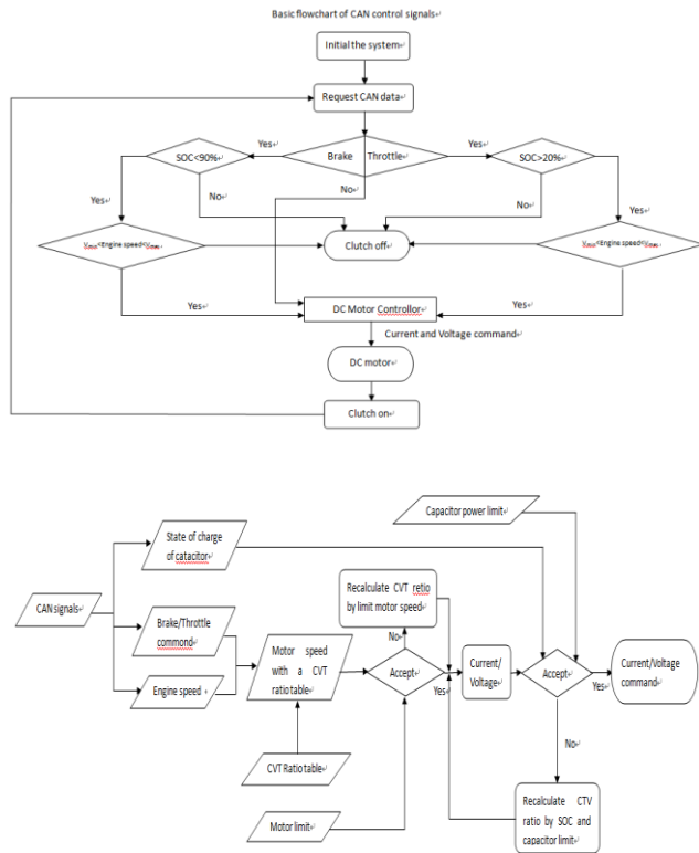
Figure.5 Hybrid plus system controller calculation priority chart
