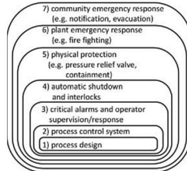
Figure 2. Independent Protection Layers
