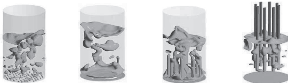
Figure 2: CFD-Simulation, investigation of 4 different reactor geometries
