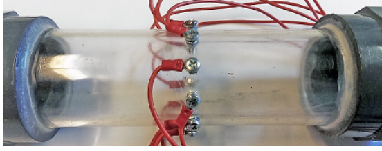
Fig. 5. Illustration of the ERT sensor configuration
