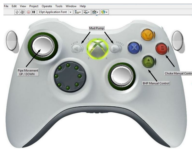
Fig. 4. Joystick Control of the Drilling Simulator
