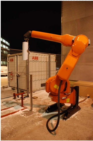
Fig. 5. The outdoor test facility enables testing in more realistic environments. Most prominently, the effect of various weather- and lighting conditions must be taken into account. To minimize the deployment gap between the outdoor tests and on-site demonstrations, an ATEX-certified ABB robot (IRB5500) is utilized.
