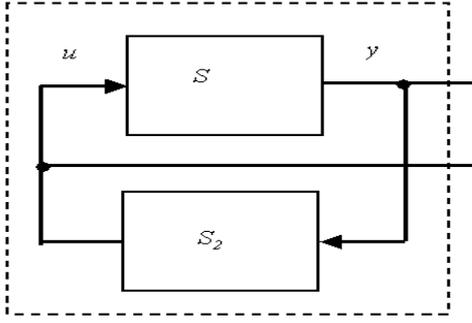
Fig. 4. General feedback control composition
