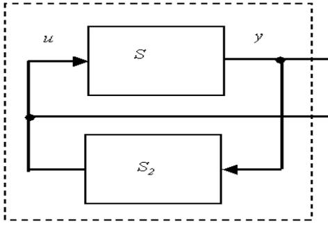
Fig. 4. General feedback control composition
