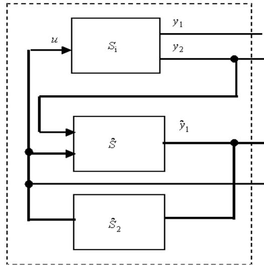
Fig. 6. State feedback with observer
