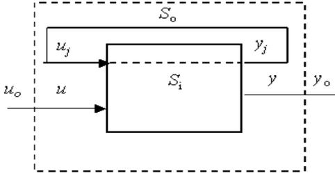
Fig. 3. General composition with free internal inputs
