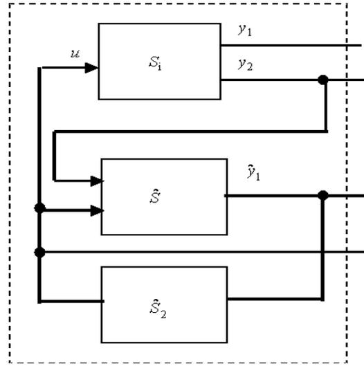
Fig. 6. State feedback with observer
