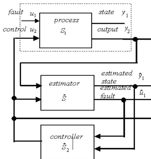
Fig. 1. Fault-tolerant control
