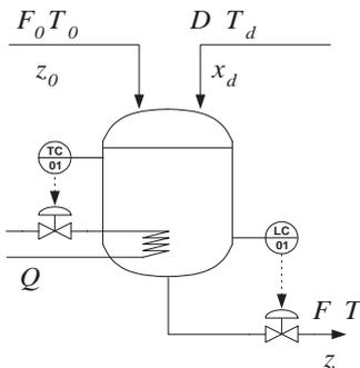
Figure 1: CSTR with first order exothermic reaction
