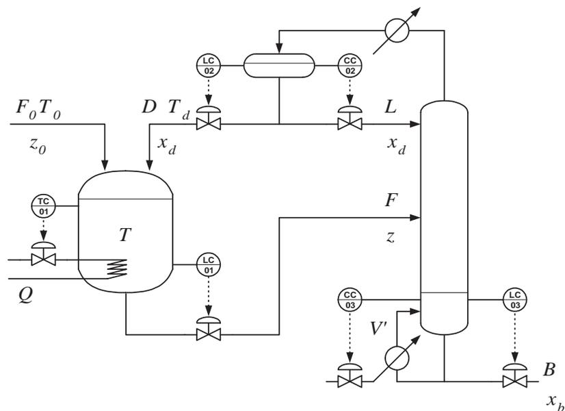
Figure 5: Reaction separation process
