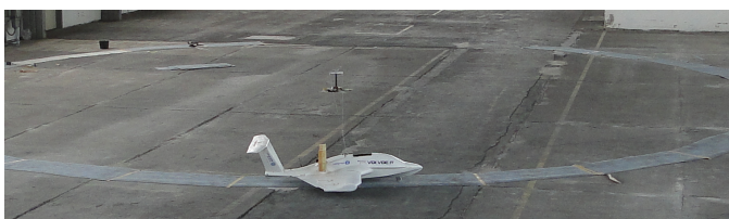
Fig. 3. Scaled WIG craft rebuilt as captive plane and tested in a large, empty storage hall
