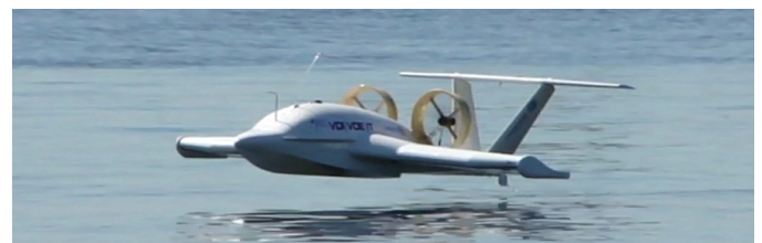
Fig. 4. Scaled WIG craft flying over water
