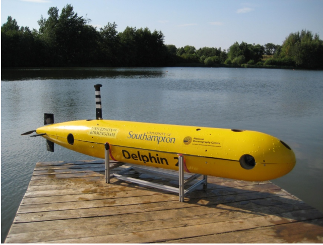
Fig. 1. Delphin2 AUV: Over-actuated hover capable AUV
