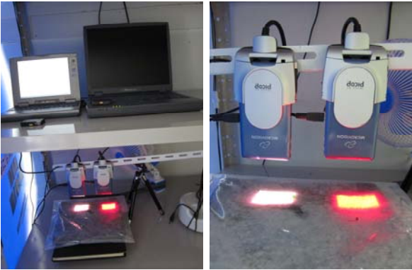
Fig. 2. Precision artificial lighting system for moss mat production using scanning type Laser Diode (LD) lighting system.
