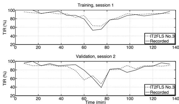
Fig. 9. Estimated and recorded TIR for IT2FLS No.3. Training and Validation.
