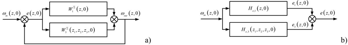
Fig. 6. Transformed block diagrams of system with wide range PWM: (a) closed-loop system, (b) equivalent open-loop system.
