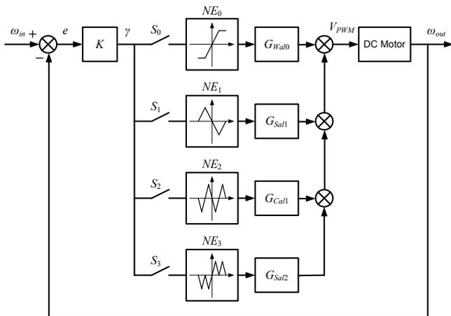
Fig. 3. Multi-channel model of stabilising system with an equivalent pulse-amplitude modulation.
