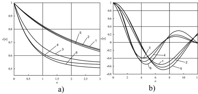
Fig. 7. Error of system control with wide range PWM for (a) proportional and (b) proportionally-integral regulators.
