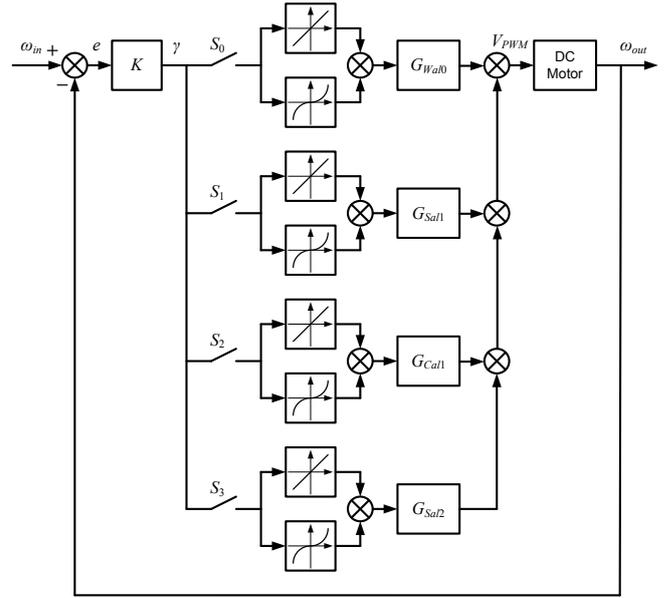
Fig. 5. Multi-channel model of system with a wide range PWM, taking into account the nonlinearities of elements.
