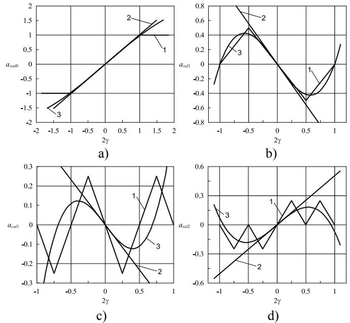
Fig. 4. The amplitude characteristics of channels of the converter model with a wide range of PWM: a)  $a_{Wal0}$  channel, b)  $a_{Sal1}$  channel, c)  $a_{Cal1}$  channel, d)  $a_{Sal2}$  channel.
