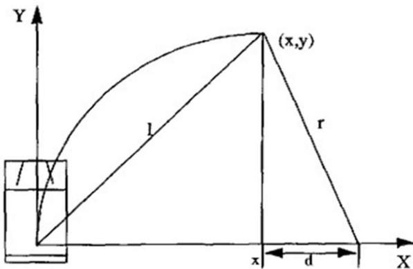
Fig. 4 Pure pursuit algorithm geometry (Coulter, 1992)
