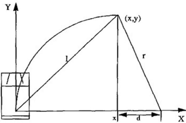
Fig. 4 Pure pursuit algorithm geometry (Coulter, 1992)
