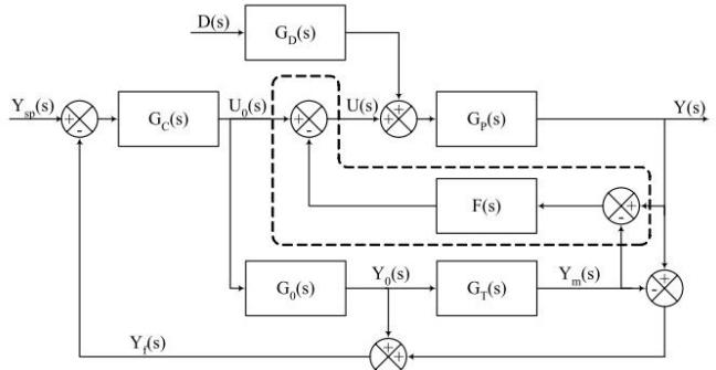
Fig. 6 The Smith-predictor structure used in this research (Rice & Cooper, 2003)
