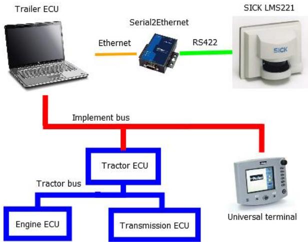
Fig. 2 Architecture of trailer coupling system
