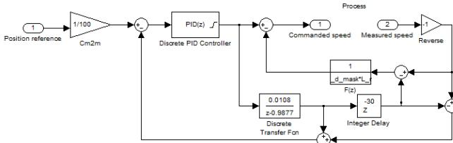
Fig. 7 The Smith-predictor used for the process
