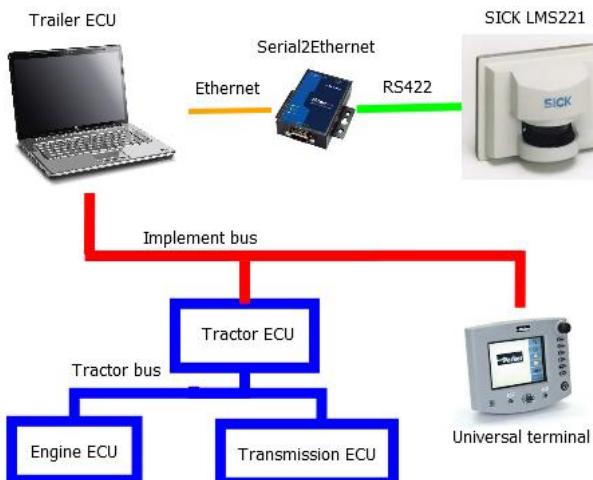
Fig. 2 Architecture of trailer coupling system
