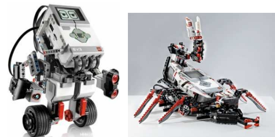
Fig. 3. An inverse pendulum designed as a biped robot and a scorpion built with NXT-EV 3 .
