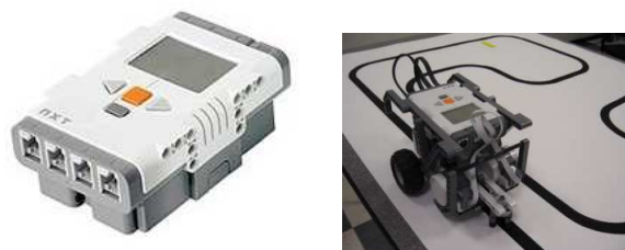
Fig. 2. A line-follower application developed with a Lego NXT differential wheeled robot.
