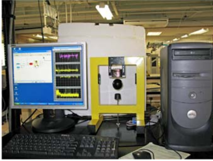
Fig. 1. A magnetic levitation system -Real System
