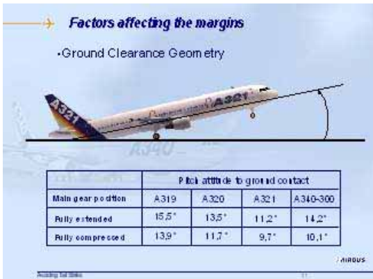
Tailstrike margins on a “geometry limited” aircraft
