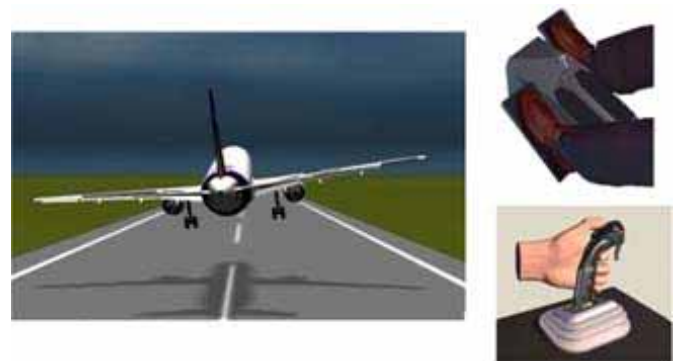
Crosswind landing technique: downwind rudder and upwind stick
