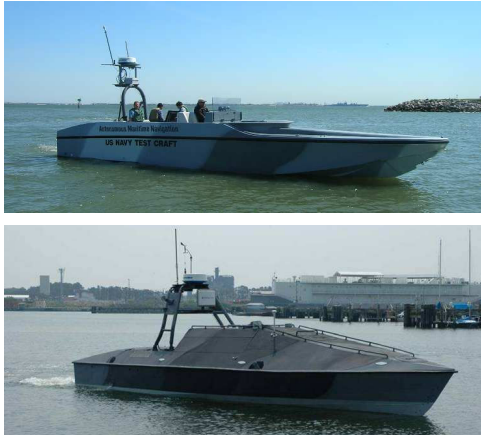
Fig. 8. USSVs used in experimental tests: Top: U. S. Navy PowerVent APTD (Advanced Propulsion Technology Demonstrator); Bottom: U. S. Navy USSV-HTF (High Tow Force).
