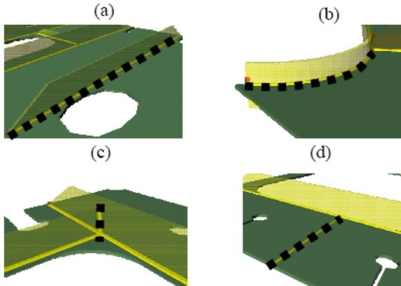
Fig. 3. Definitions of seam line: (a) horizontal linear fillet joint, (b) horizontal linear circular joint, (c) vertical linear fillet joint and, (d) horizontal linear butt joint
