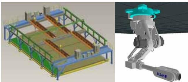
Fig. 4. Robot gantry and manipulator
