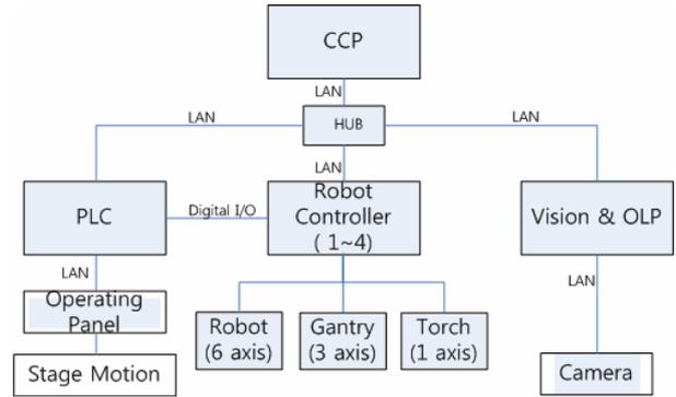
Fig. 12. Control structure of CCP
