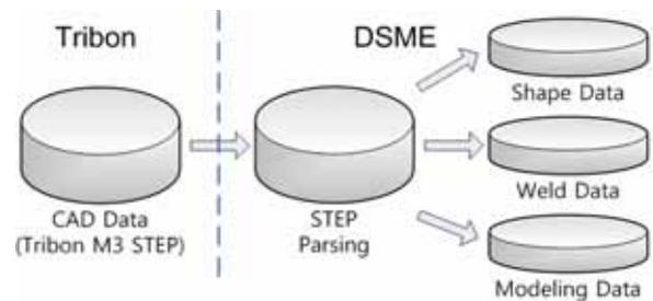
Fig. 5. Procedure of CAD Data Interface
