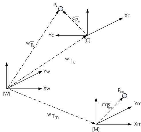
Fig. 9. Transformation between CAD data and work pieces
