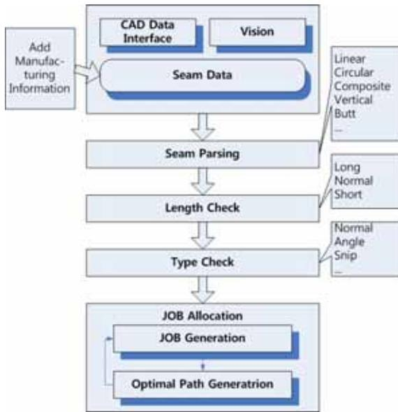
Fig. 11. Flow chart of robot program generation
