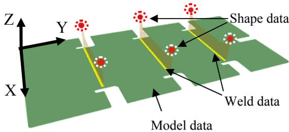
Fig. 6. Example of Shape data, Weld data and VRML data
