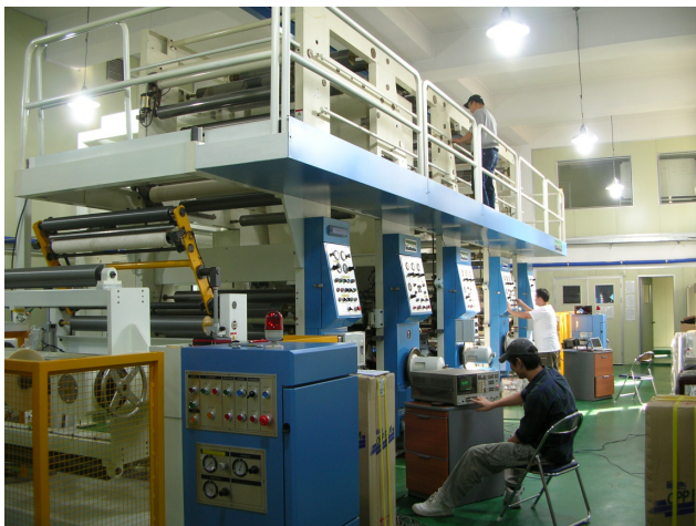
Fig. 2 Pilot gravure printing machine installed at FDRC at Konkuk University (Courtesy of SAM, Inc. and FDRC).
