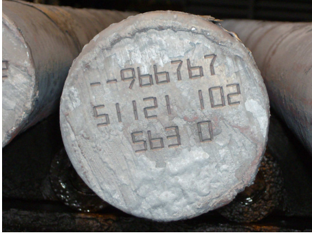
Fig. 3. Example of Hammer marked characters.
